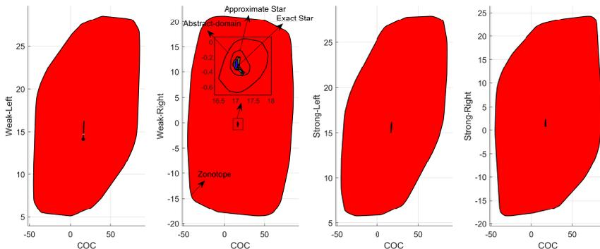
(b) Reachable sets of  $N_{3.8}$  network w.r.t property  $\phi_3$  with different methods. The zonotope (used in DeepZ [20]) and abstract-domain (used in DeepPoly [21]) methods cannot verify the property due to large over-approximation error.
