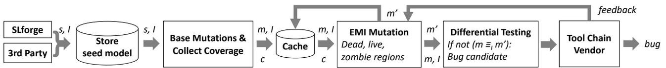
**Figure 2: Overview: SLEMI first obtains seed model  $s$  with input vector  $l$  from a real-world corpus or a random generator (e.g., SLforge), performs one-time base mutations to yield model  $m$ , and collects  $m$ 's coverage  $c$  (on  $l$ ). An EMI-based mutation then yields a valid equivalent (on  $l$ ) model  $m'$  (i.e.,  $m \equiv_l m'$ ) for finding tool chain bugs via differential testing. [3]**
